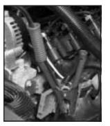
The remote positive (+) terminal is located near the engine accessory drive bracket. On some vehicles, the terminal may be covered under a red plastic cover. To access the remote positive (+) terminal, open the red plastic cover.
